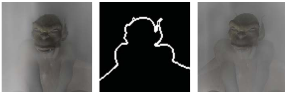
Figure 30-22. Fixing Artifacts Introduced by Low-Resolution Off-Screen Rendering Left: Ray marching at a low resolution and upsampling can cause artifacts near sharp silhouettes. Center: Detecting these features and rendering the corresponding fragments at higher resolution. Right: The resulting artifact-free image.
