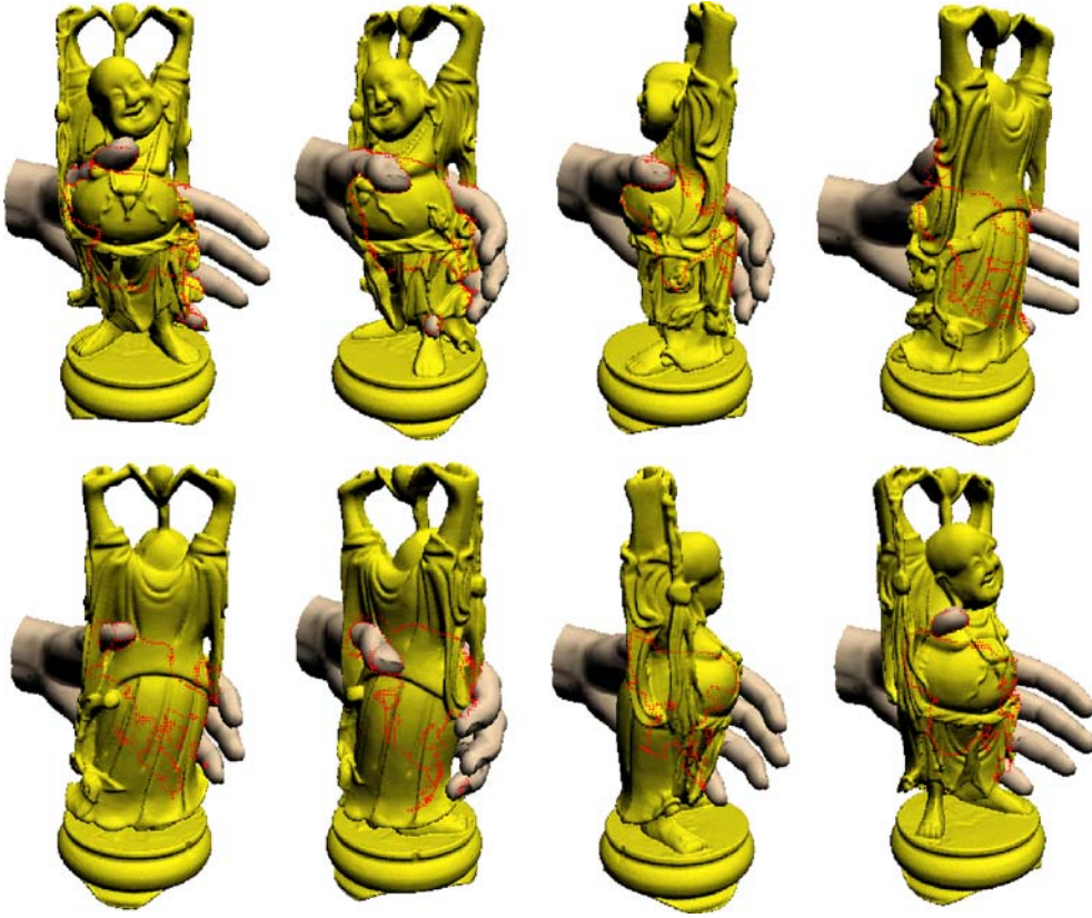
Fig. 8. Interactive collision detection based on conservative voxelization
